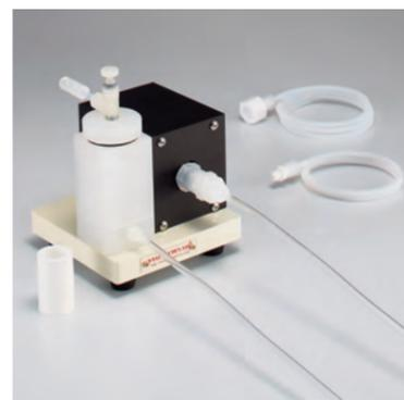
A filter able to be used for tanks with small volume (300 - 1000mL), such as beakers. Normally PVC tubes are included. Exchangeable to separately sold PTFE tubes.
