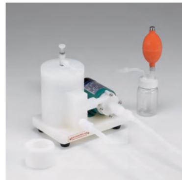
PTFE tube-filter with excellent heat-resistant and chemical-resistant properties. Used for small volume (approx. 1L) of solution.
