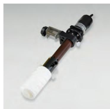
Filtering and agitation equipment can be used for 95°C electroless plating. Since its motor and propeller are apart and do not disturb cooling function, also can be used for anodizing. Activated carbon filtration is also possible. Applied to tanks of approximately 10 - 100L volume.
